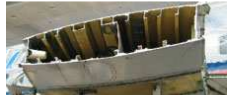
This cross section of an airplane wing shows the similarity to Lund construction methods: Longitudinal I-beams and Z-beams form a strong, rigid structure, fastened with the highest-quality riveting.
